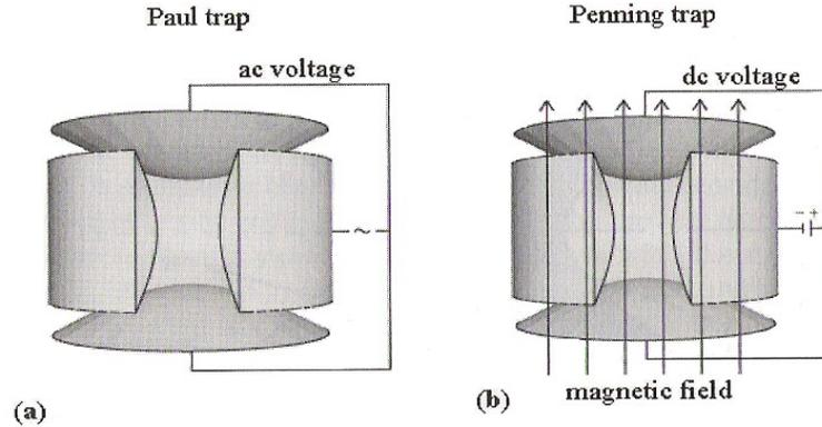
Figure 1. Basic arrangement for Paul and Penning traps. The inner electrode surfaces are hyperboloids. (a) The dynamic stabilization in the Paul trap is given by the ac-voltage  $V_0 \cos \Omega t$ ; (b) The static stabilization in the Penning trap is given by the dc-voltage  $U = U_0$  and the axial magnetic field  $B$  (Figure reproduced from [4])
