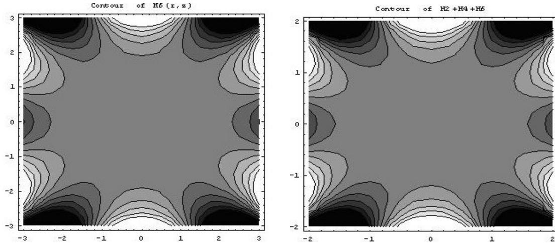
Figure 2. Surface contours for the quadrupole, octopole and dodecapole terms of the potential and for a linear combination of them
