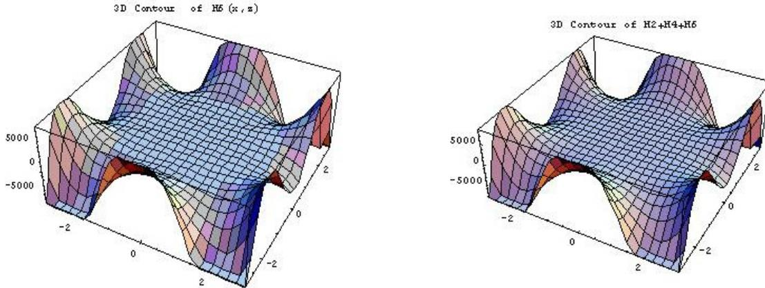
Figure 3. Space (3D) contours for the quadrupole, octopole and dodecapole terms of the potential and linear combinations of them
