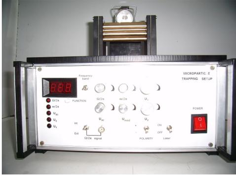
Figure 4: Microparticle confinement setup based on a hexapolar trap geometry, operating in air, at standard temperature and pressure conditions.
